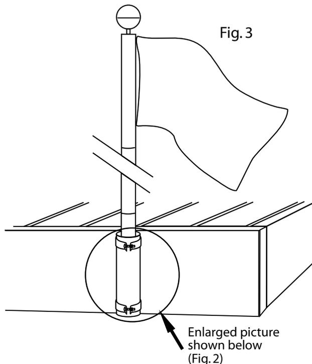
1. Drill a 1/4" hole in PVC sleeve approximately 1/2" from the bottom end of the sleeve on both sides. Insert a 1/4" carriage bolt through hole and fasten securely with a nut. Bolt serves as a stop bolt to support pole within sleeve. (See Fig. 2)
